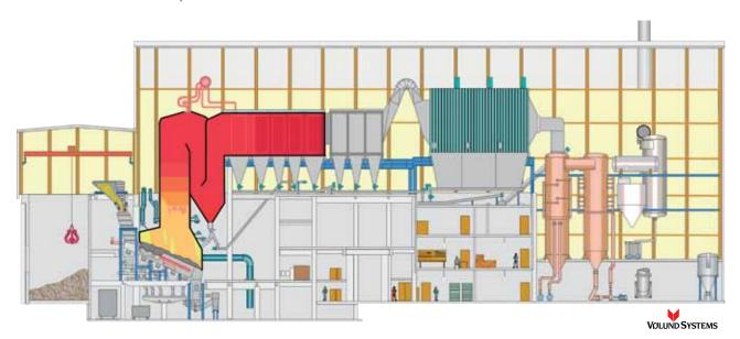
The nominal capacity of the plant is 20 t/h waste at a calorific value of 12 MJ/kg, corresponding to approx. 160,000 t/year. The boiler generates 80 t/h steam at 50 bar, 425°C.
