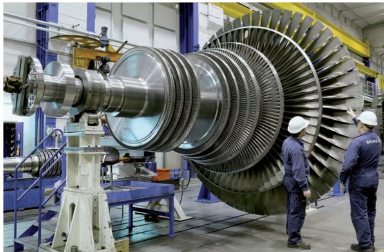
The LP rotor under assembly in the Swedish workshop. The diameter of the last stage blades is the largest fabricated for this type of turbine.
